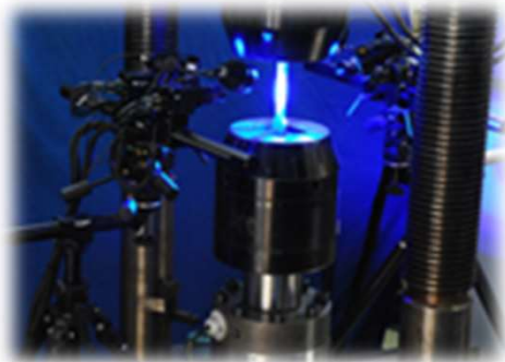
Monitoring of progressive fatigue damage with ARAMIS 3D DIC
