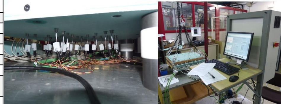
Permeability test rig for composites developed in ITAINNOVA.
