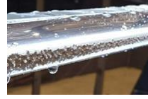
Anti-ice + Hard Hydrophobic → Anti-ice wings and lead erosion resistant blades.
